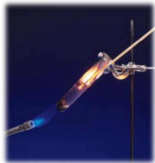
Heating potassium chlorate produces oxygen, which supports the combustion of wood splint.
